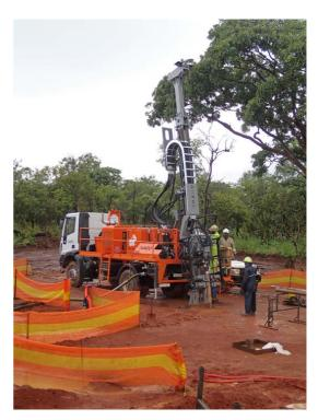
ous, relatively undisturbed in-situ core sample in soft or broken ground – it is best used for lithium and tailings pile testing.
