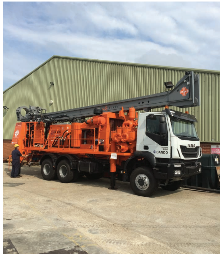
Mounted as standard on a 6 x 6 or 8 x 8 truck for quick mobilisation between sites of long distance.
