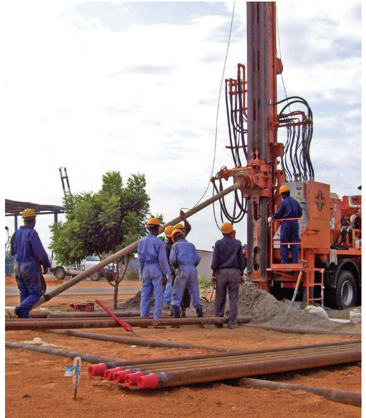
High torque rotary head with hydraulic side shift and head tilt.
