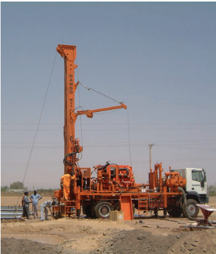
Features include main winch for tools and casing; auxiliary winch for tool handling; a selection of on-board air compressors and mud pumps; complete tooling packages and training available.
