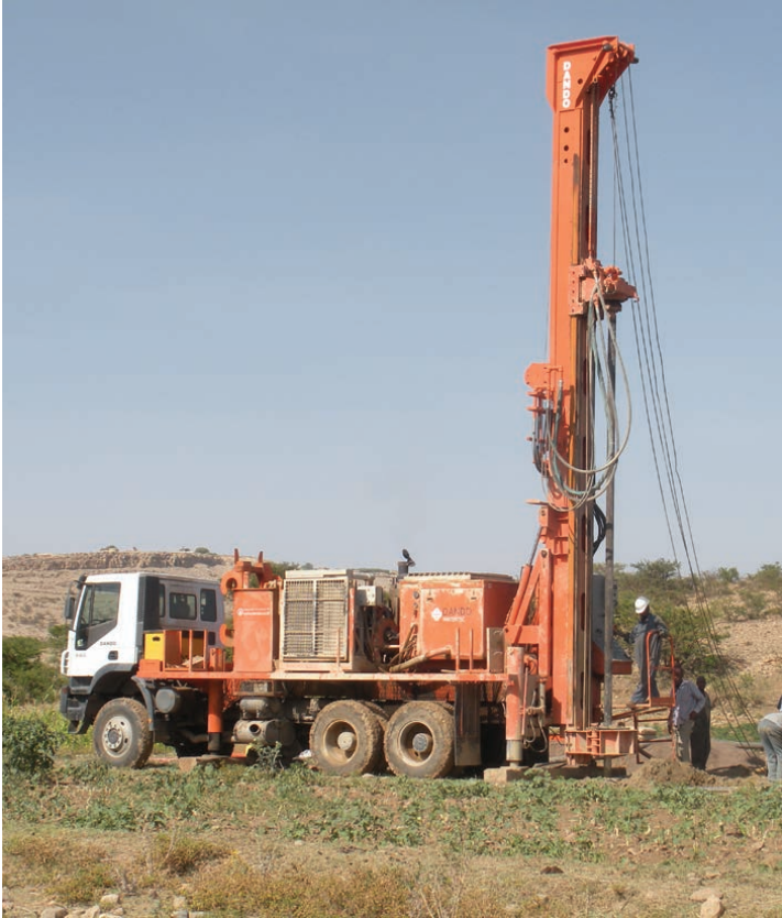
Capable of mud rotary, air and flooded reverse drilling techniques to great depths.
