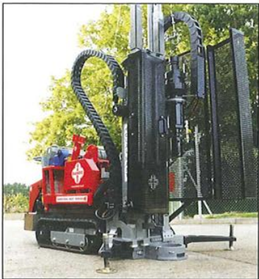
Above: the ► CORING dual-mast Terrier has both a percussive mast and a rotary mast
