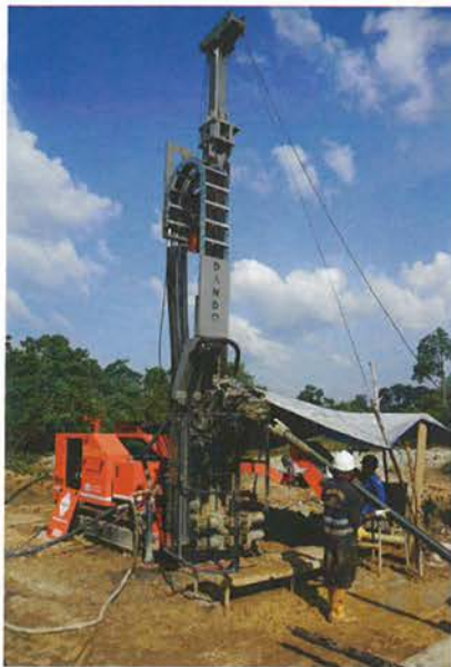
Coring for coal in Indonesia: the Multitec 9000 is modular, allowing exploration teams to choose components to suit their project and budget.
