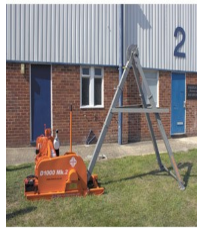
The Dando 1000 MK2 features an adjustable height mast derrick. Source: Dando Drilling International
