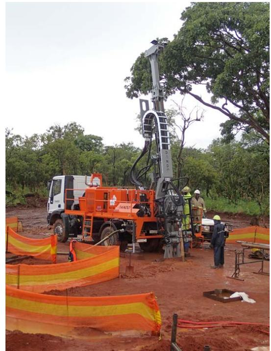
ous, relatively undisturbed in-situ core sample in soft or broken ground – it is best used for lithium and tailings pile testing.
