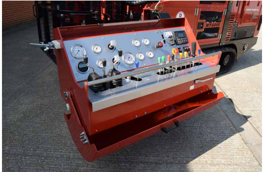
The control panel is mounted on a sturdy swing-out arm to give the operator a clear view of the borehole. Controls are clearly laid out and well spaced for easy operation.
